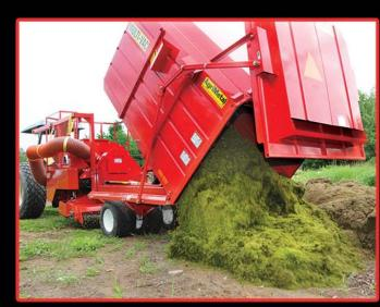
A hydraulic dump system is used to empty the debris from the hopper. The hopper tilts up to a 60 degree angle to completely empty the box. This system is quick and efficient allowing the operator to return to the field, thus maximizing productivity.
