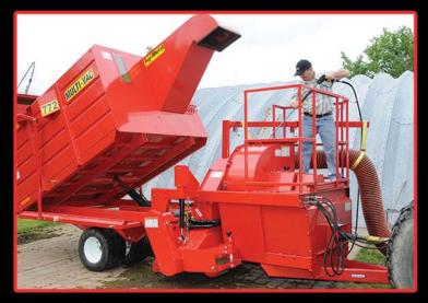
A platform located around the blower housing enable the operator to safely & properly clean out the inside of the blower. A drain trap is located at the bottom of the blower to drain water and residues. Once the hopper is tilted, it is quick and easy to wash out the inside.
