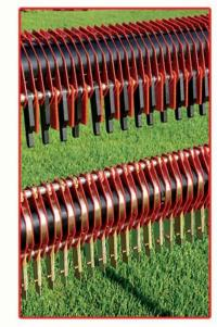
AgriMetal has developed a new brush system that is second to none in sweeping leaves and branches. The brush is made of 3/8" wide high-strength nylon fingers with shorter steel knives located between the nylon fingers. The nylon fingers and steel knives are made to freely pivot so as not to damage the turf, while throwing leaves and branches into the intake.
